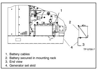
Figure 7-1 Typical Battery System, Side View
